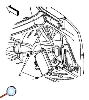
**Important:** The vehicle communication interface module (VCIM) has a specific set of unique numbers that tie the module to each vehicle. These numbers, the 10-digit station identification and the 11-digit electronic serial number, are used by the National Cellular Network and OnStar® to identify the specific vehicle. Because these numbers are tied to the vehicle identification number of the vehicle, you must never exchange these parts with those of another vehicle.
